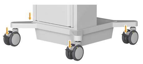
> Lock all four caster wheels with the brakes when the cart is in the required position.
